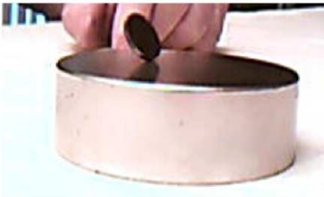
FIG. 3: RTS disk of a diameter about 2 cm and about 3.4 mm thick is on the surface of a 3 inch diameter permanent magnet with a B \simeq 1.4 T field in the center.
