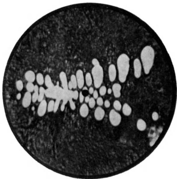
Fig. 24. — \text{Cu}_2\text{O} inclusions in copper. {}_{63}\text{Cu}^+ image (Slodzian). Magn.: 400 \times . (Courtesy of Ann. de Phys. )
