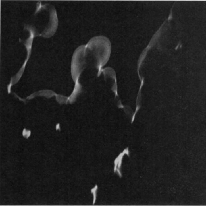
Fig. 11. – Fresnel fringe (underfocused) around carbon black particles. Inelastic image (5.9 eV loss of carbon). Magnification 150\,000\times (Henry). (Courtesy of Compt. Rend. Acad. Sci. Paris. )
