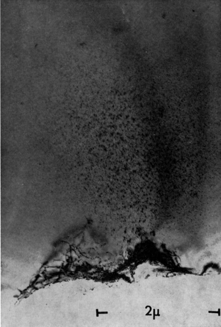
Fig. 17. - The distribution of loops within the electron irradiated spot.
