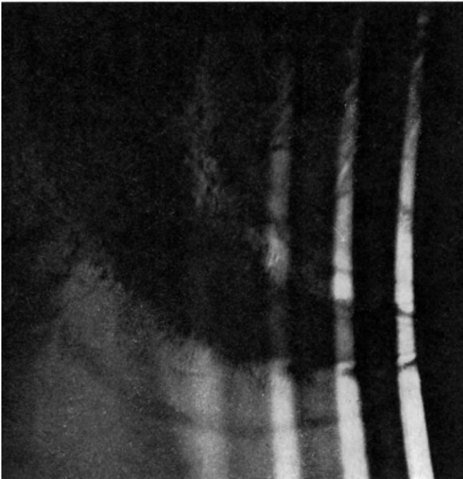
Fig. 16. - Extinction contours (aluminium) with superimposition of the energy loss spectrum. Magnification 30000\times (El Hili). (Courtesy of the Journ. de Microscopie .)
