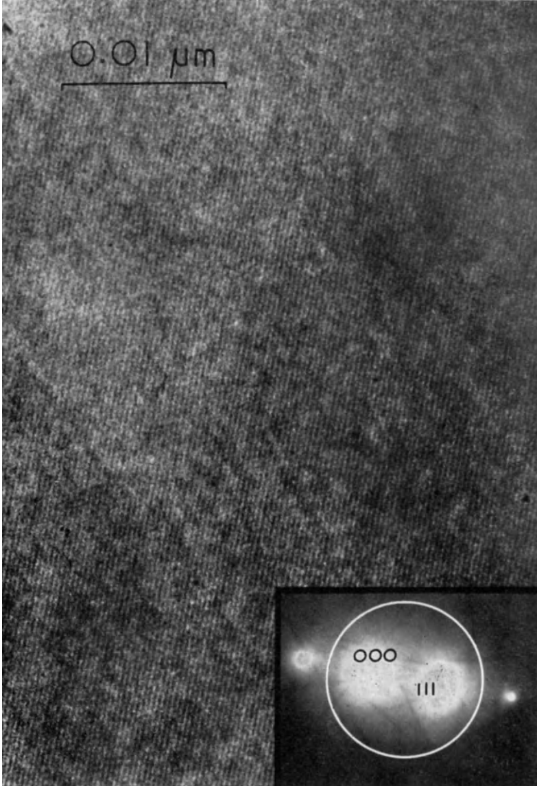
Fig. 15. – Micrograph taken using objective aperture of size and position as in inset diffraction pattern (correctly oriented).
