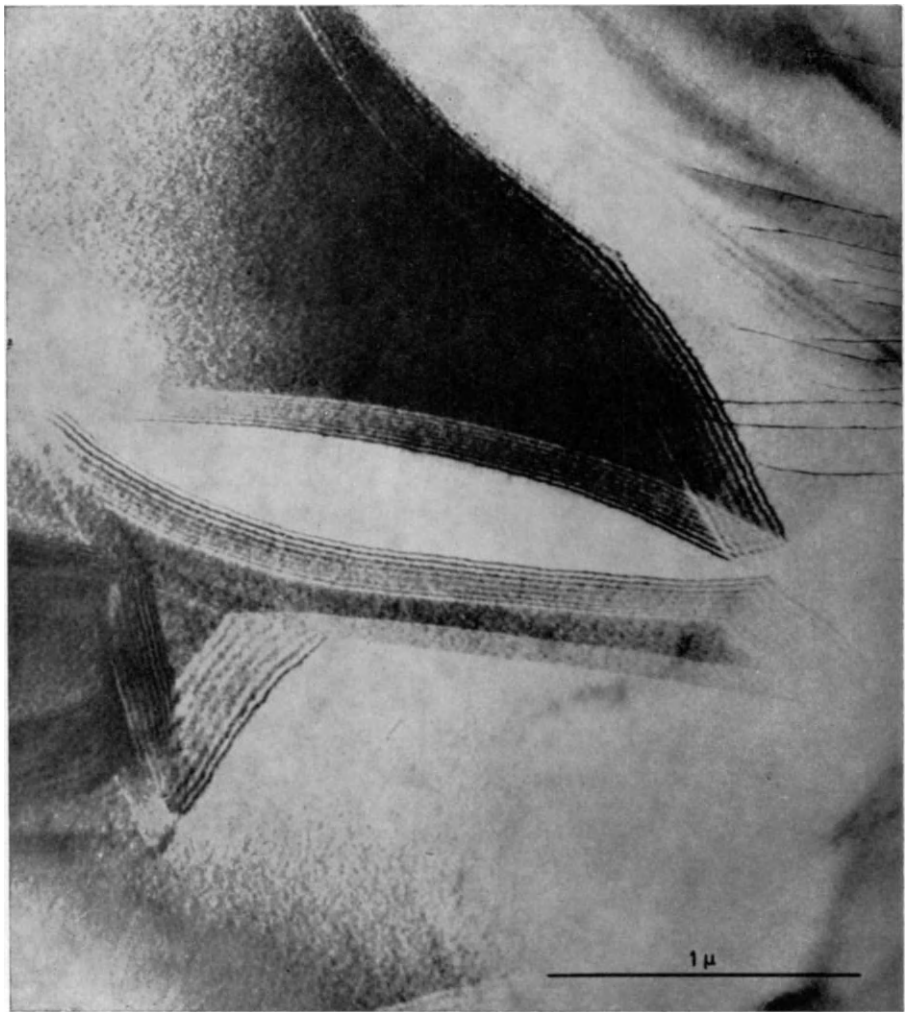
Fig. 17. – Ordered domain boundaries in Nb containing impurities. Note the difference in background in the different domains (bright field image). (Courtesy of Phys. Stat. Sol. , 5 , 595 (1964).)
