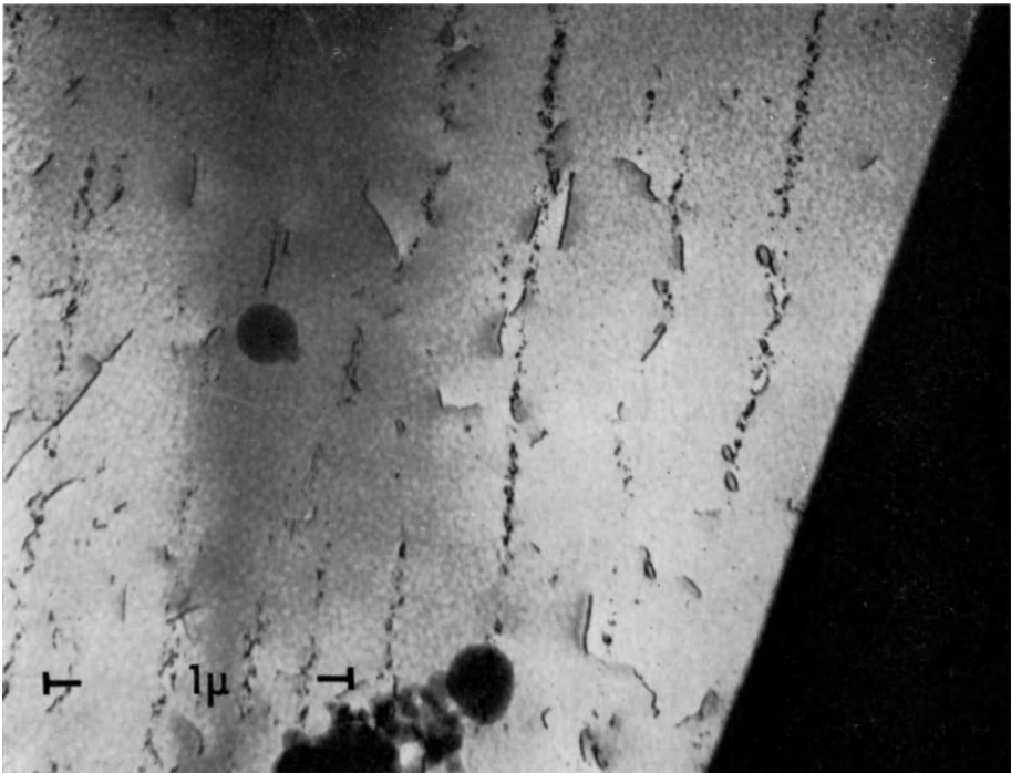
Fig. 8. – Loops aligned in sheets after irradiation at 350 °C to 1.5 \cdot 10^{17} \text{ n} \cdot \text{cm}^{-2} . (Courtesy of Phil. Mag. )
